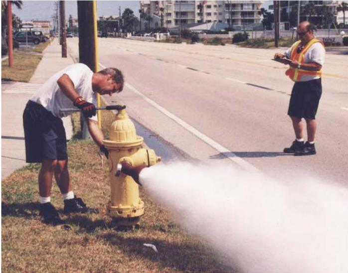
Firefighters Todd Burnett and Dave Murtha test a fire hydrant to ensure that there is sufficient flow and that all of the fittings work should the hydrant be needed. All 86 hydrants in Town are annually tested with deficiencies reported to Melbourne water.
