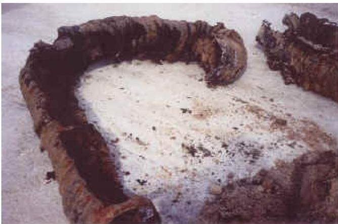
The Town's closed storm drain system, installed 40 years ago, consists of approximately 38,000 linear feet, or seven miles, of single coated metal pipe. Most of it needs to be replaced. The replacement cost estimate is \$3.07 million.
